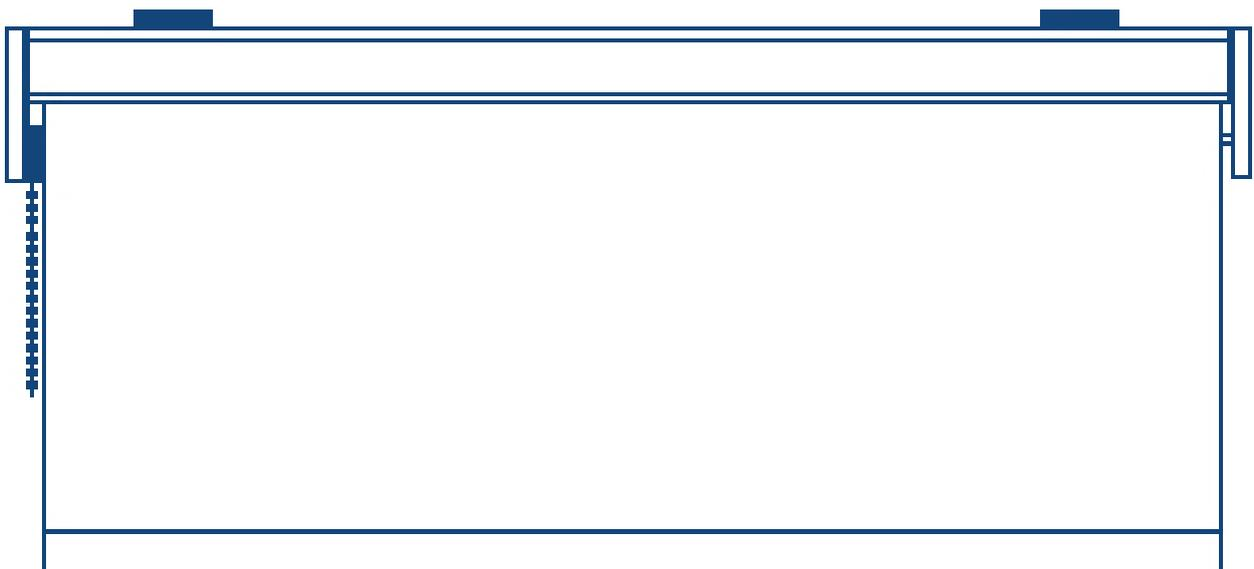
Using the pencil, mark where you're looking to fix your brackets. Remember, wherever you place them, be it top or face fitting, the outermost brackets must be 5cm away from the end of the rail.
